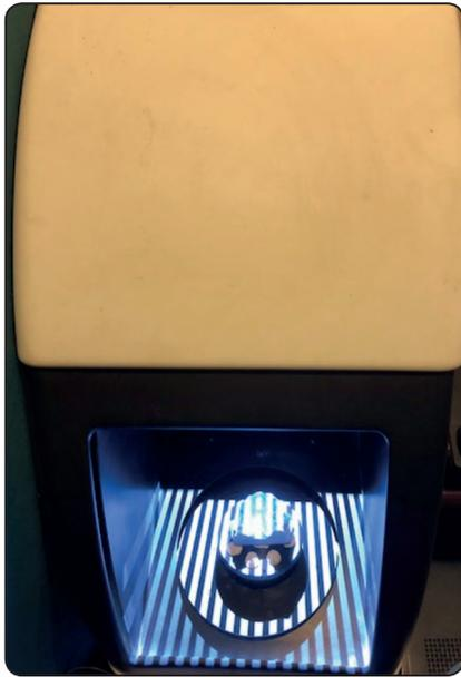
Fig. (2) Optical Scanner – Open Technologies while scanning a dental model
