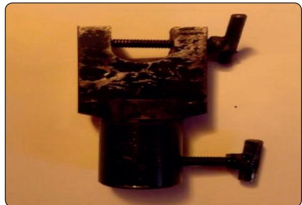
Fig (5) Showing Two custom made metallic hooks were fabricated to be fixed to the upper and lower parts of the Instron machine.
