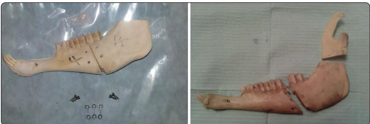
Fig. (2) Showing condylar process were removed to avoid difficulty of fixation on the test jig during load application
