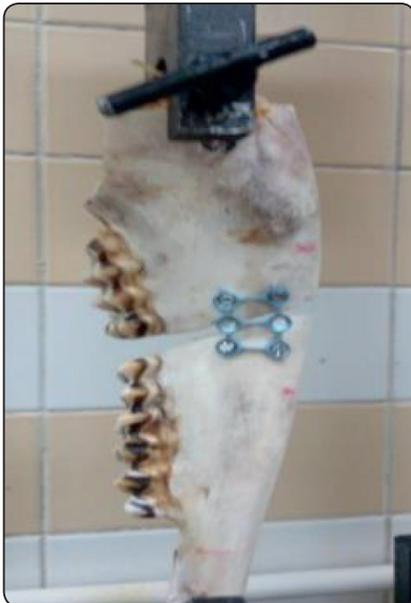
Fig (6) Showing The custom made tension test device was attached to the testing machine and was used for compression test for Group (2) prepared samples.
