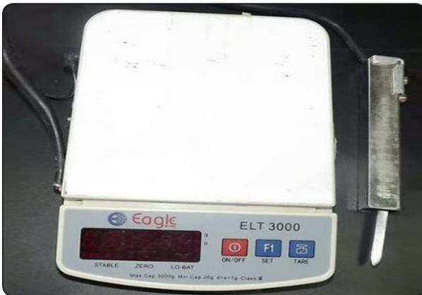
Fig. (1) Digital force meter used in the study
