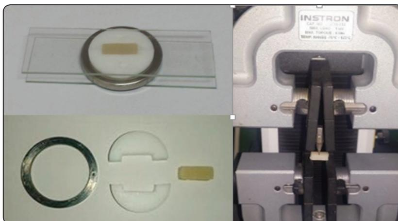
Fig. (1) Preparation and testing of the specimens.
