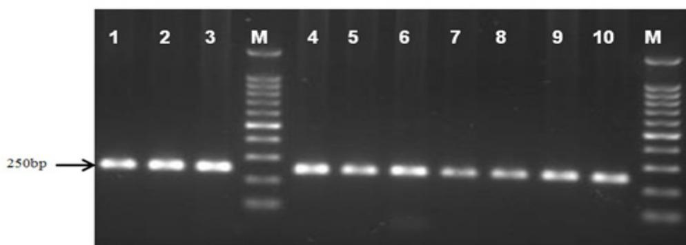
Fig.1. PCR product of OPN gene (250 bp) visualized on 1.5% agarose gel. M= 100 bp. Molecular marker Lanes 1-10 resemble PCR products
