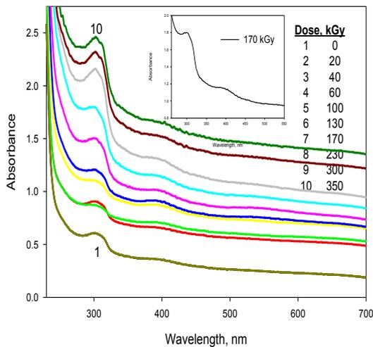
Fig. 1. UV/Visible spectra of the unirradiated and irradiated PVA/PVP/Ni composite films (0.015M) at different doses
