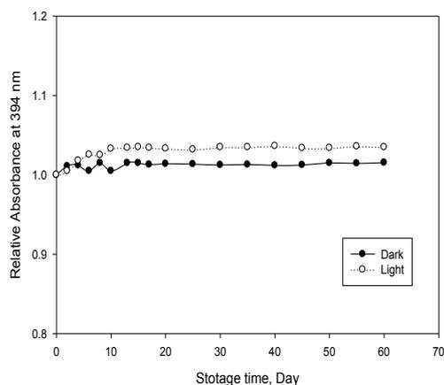
Fig. 5. Post-irradiation stability of PVA/PVP/Ni<sup>0</sup> nanocomposite in the dark and light at room temperature
