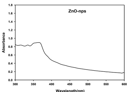
Fig. 3. UV-vis of ZnONPs
