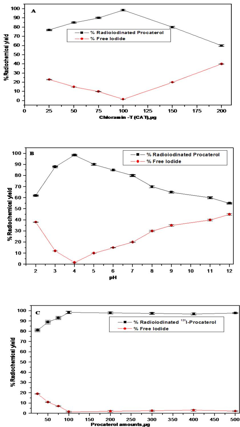
Fig. 3. Variation of the radiochemical yield of radioiodinatedprocaterol as a function of Ch-T amount (A), pH (B), procaterol amount (C) and reaction time (D)
