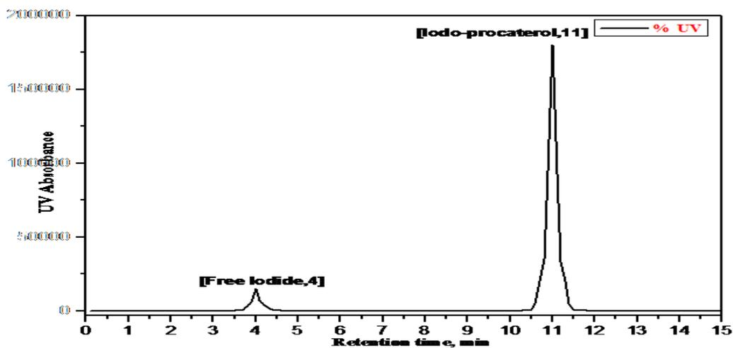
Fig. 2b . HPLC U.V. absorption chromatogram of the reaction mixture of procaterol and KI using Ch-T as oxidizing agent.
