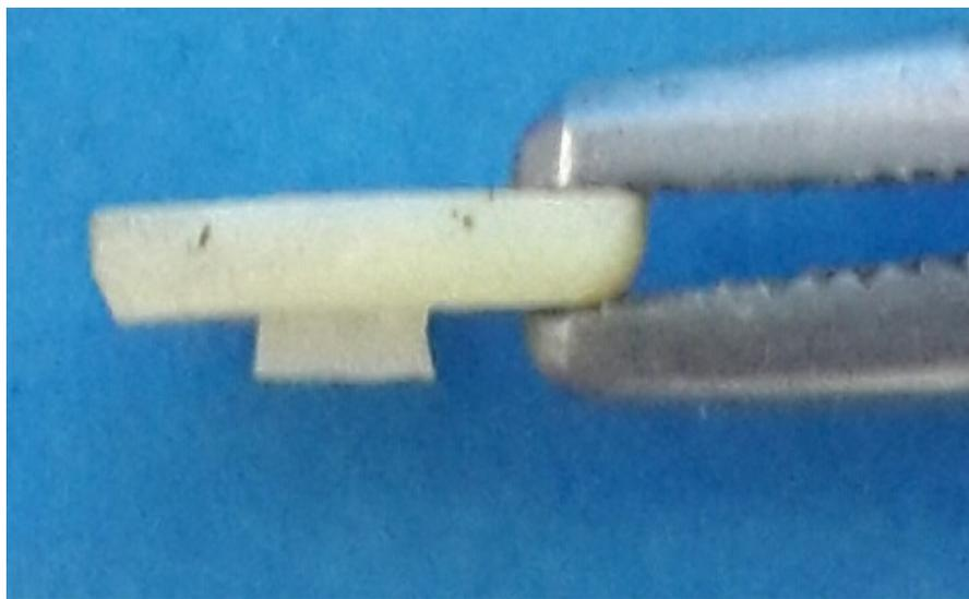
Fig. 1. The failure reported on extrusion of the restoration from the prepared specimen.
