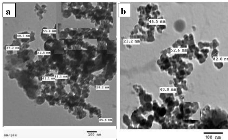
**Fig. 3. TEM images of (a) CS50VC and (b) CS100VC.**
