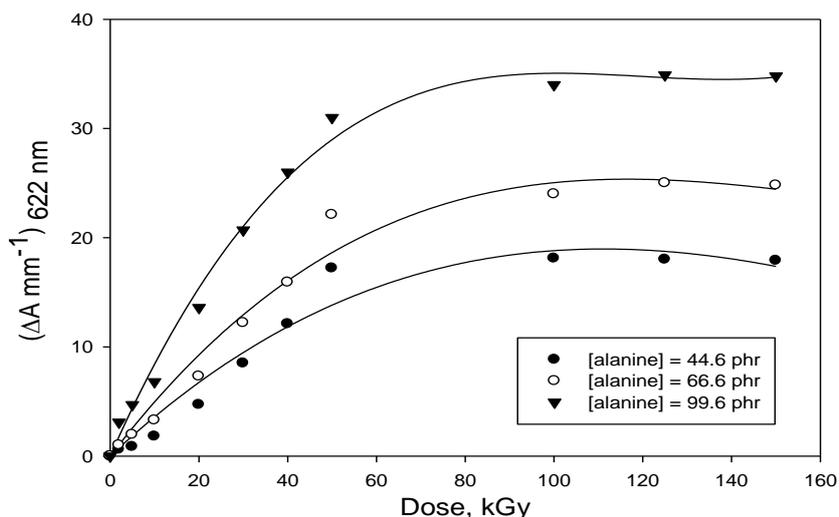
Fig. 3. Change of absorbance at 622 nm as a function of absorbed dose of (BTB-MO)/PVA films with different concentrations of  $\alpha$ -alanine.
