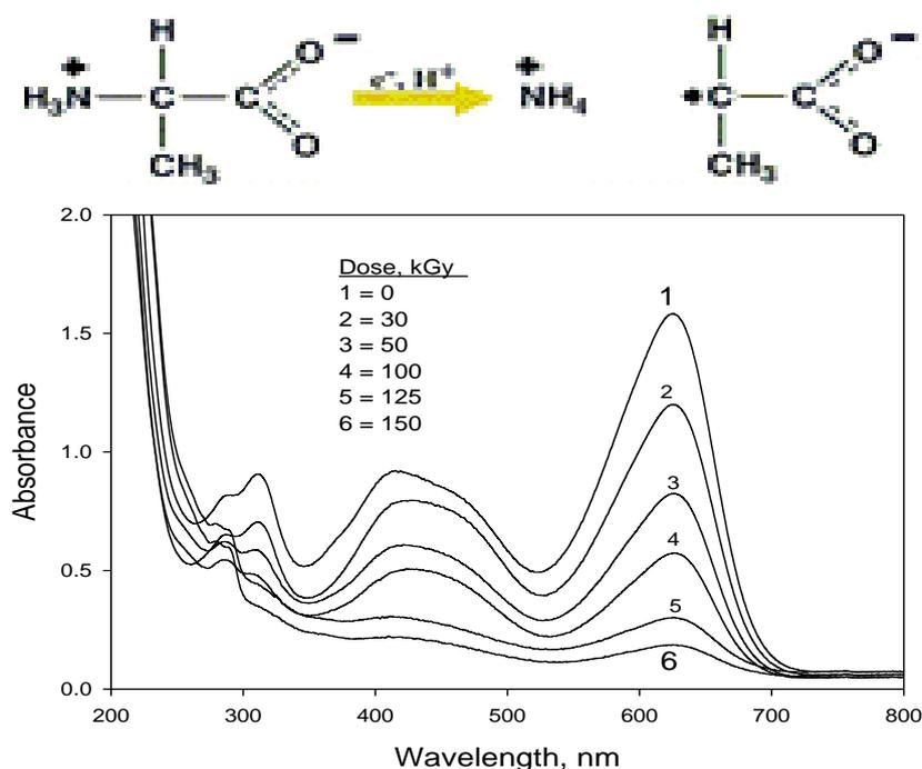
**Fig. 2.** The absorption spectra of (BTB-MO)/ PVA films unirradiated and irradiated to different absorbed doses. [ $\alpha$ -alanine]= 66.6 phr.
