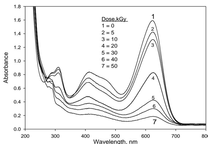
**Fig. 1.** The absorption spectra of (BTB-MO)/ PVA films unirradiated and irradiated to different absorbed doses.
