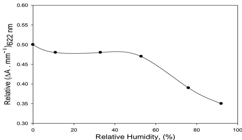
**Fig. 4.** Variation of response of (BTB-MO)/ PVA films (at 622 nm) as a function of relative humidity during irradiation, where response in  $\Delta A \cdot \text{mm}^{-1}$  at 30 kGy.
