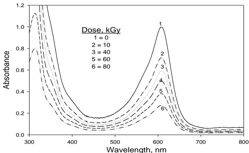
**Fig. 1. The absorption spectra of TBPE/ PVA films unirradiated and irradiated to different doses.**
