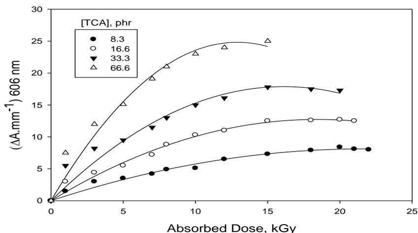
**Fig. 4.** Change of  $\Delta A. \text{mm}^{-1}$  as a function of absorbed dose of TBPE/PVA films with different concentration of tri chloro acitamide, [TBPE]= 0.66 phr.
