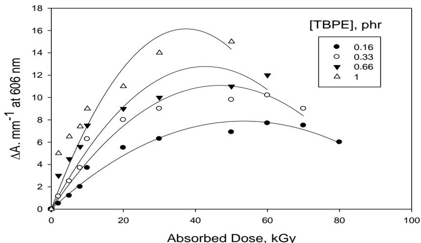
**Fig. 3.** Change of  $\Delta A. \text{mm}^{-1}$  as a function of absorbed dose of TBPE/ PVA films with different concentrations of TBPE.
