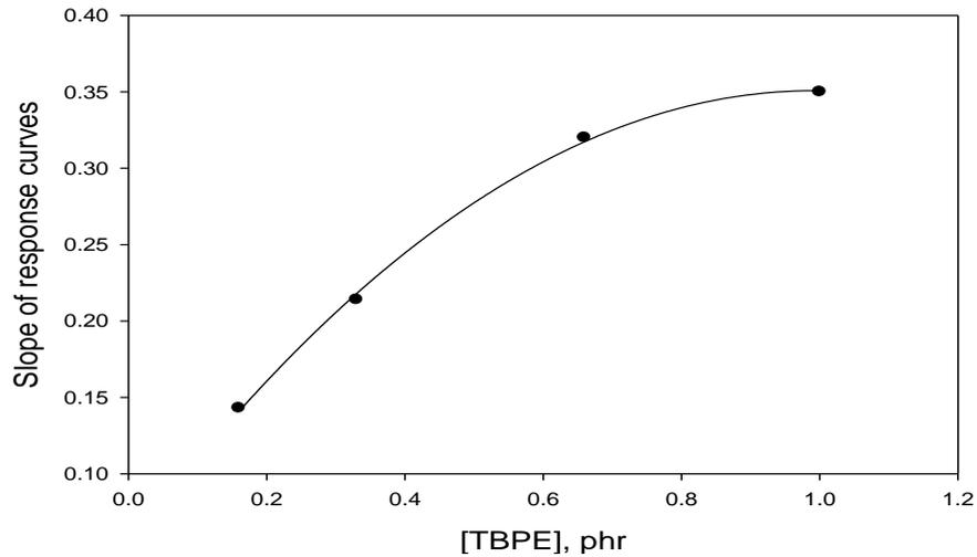
**Fig. 5. Radiation sensitivity of TBPE/PVA films against the concentration of TBPE.**
