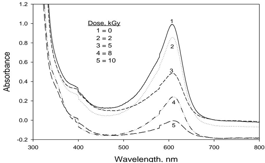
**Fig. 2.** The absorption spectra of TBPE/ PVA films unirradiated and irradiated to different doses [TCA]= 0.4 phr.
