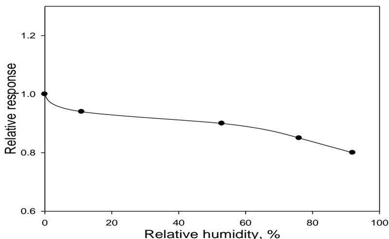
**Fig. 6.** Variation of response of TBPE/PVA films as a function of relative humidity during irradiation where response in  $\Delta A.\text{mm}^{-1}$  at 5 kGy. [TBPE]= 0.66 phr.
