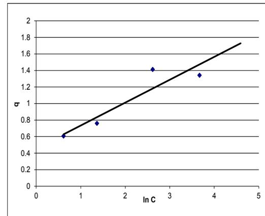
Fig. 11. Temkin plot of lead adsorption by BLB.
