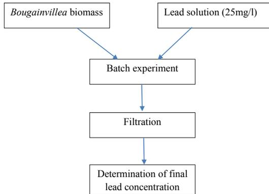
**Fig. 2. Schematic representation of the experiment.**
