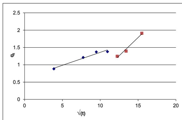
Fig. 7. Intra-particle diffusion mechanism of lead adsorption by BLB.
