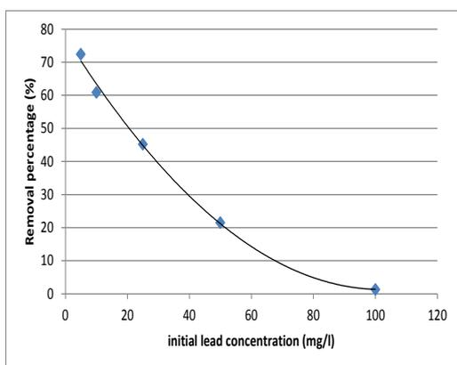
Fig. 8. Effect of lead initial concentration on its removal by BLB at contact time 90min, initial solution pH 4.5 and biomass loading weights 8g/L.
