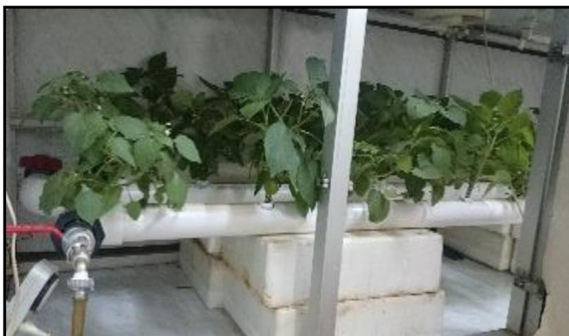
**Fig. 1. Photo of the hydroponic system, the treatment solutions in the upper water tank (inlet) transferred through the three pipes into the lower water tank controlled by a timer switch. The solution in the lower tank was drained to the upper water tank to complete a water cycle [There were one water cycles every 24 hrs].**
