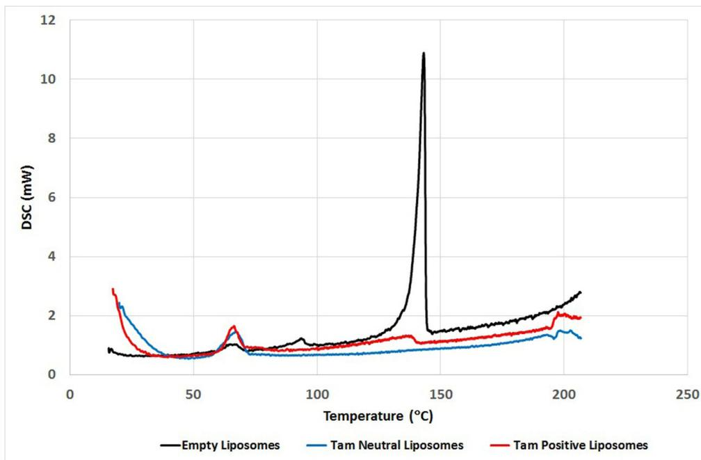
Fig. 4. DSC diagrams of liposomes made of pure DSPC and neutrally or positively charged liposomes doped with Tamoxifen.
