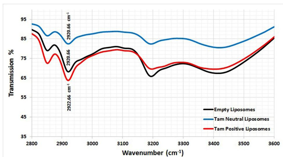
Fig. 5. The magnified part (3500–2800 cm<sup>-1</sup>) of FTIR spectra of empty DSPC and DSPC/ Tamoxifen in different liposomal formulations.
