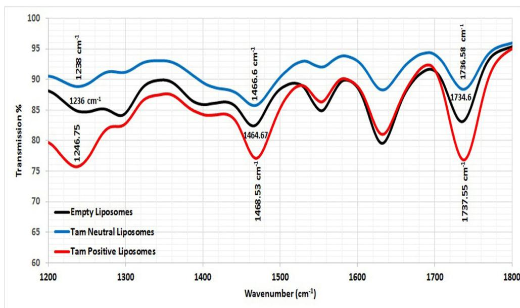
**Fig. 6.** The magnified part (1800–1200  $\text{cm}^{-1}$ ) of FTIR spectra of empty DSPC and DSPC/ Tamoxifen in different liposomal formulations.
