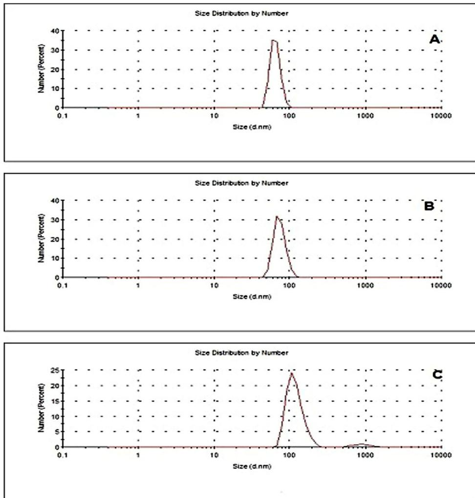
**Fig.3.** Liposomes size distribution measured by dynamic light scattering (DLS) for (A) empty liposomes (B), Tamoxifen-loaded neutral liposomes and (C) Tamoxifen-loaded positive liposomes.
