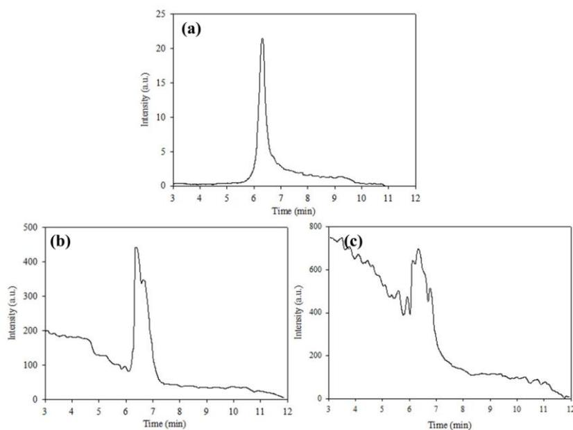
**Fig. 1. Chromatogram of the standard PC (a), hen egg yolk phospholipids (b), duck egg yolk phospholipids and (c) (Mobile phase, methanol; flow rate, 1.0 ml·min<sup>-1</sup>; column temperature, 30 °C; sample injection, 10, 20 and 40  $\mu$ l, respectively).**
