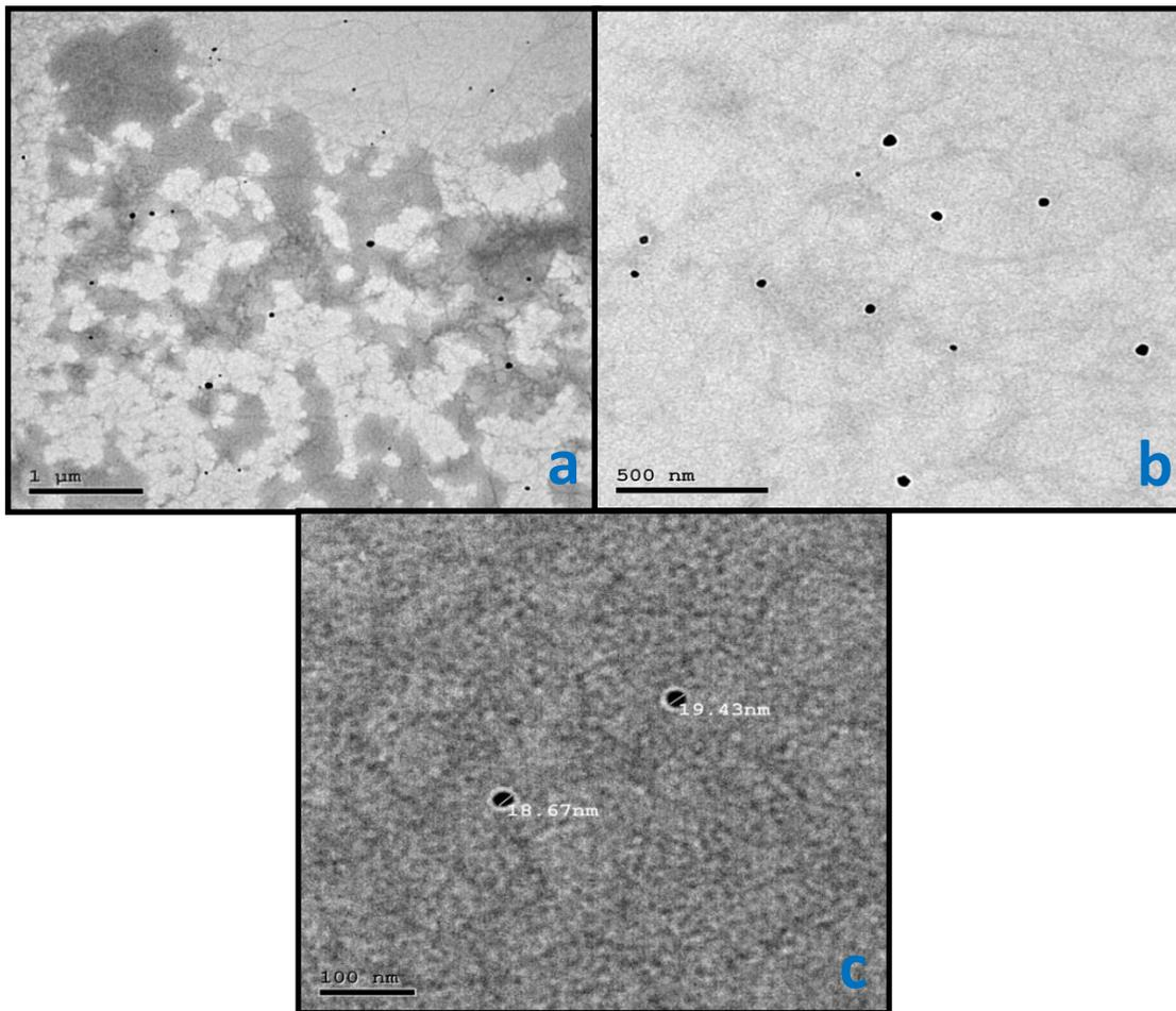
Fig 5. TEM images of CS-AgNPs with scale bars of a) 1.0  $\mu\text{m}$ , b) 500 nm and c) 100 nm
