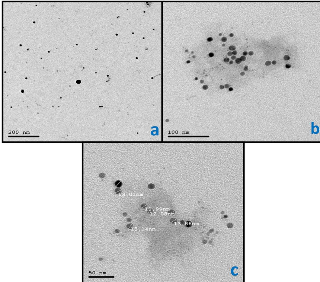
**Fig 3.** TEM images of MHB-AgNPs with scale bars of a) 200 nm, b) 100 nm and c) 50 nm
