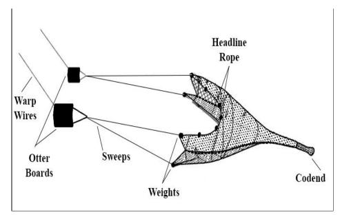
Fig. 2. Bottom trawls and their parts that work in the fisheries of the Gulf of Suez.
