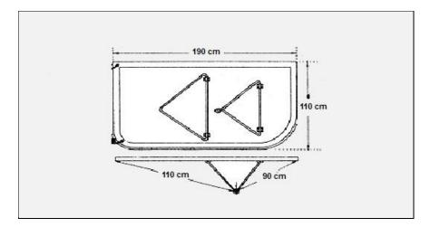
Fig. 3. General structure of otter board.
