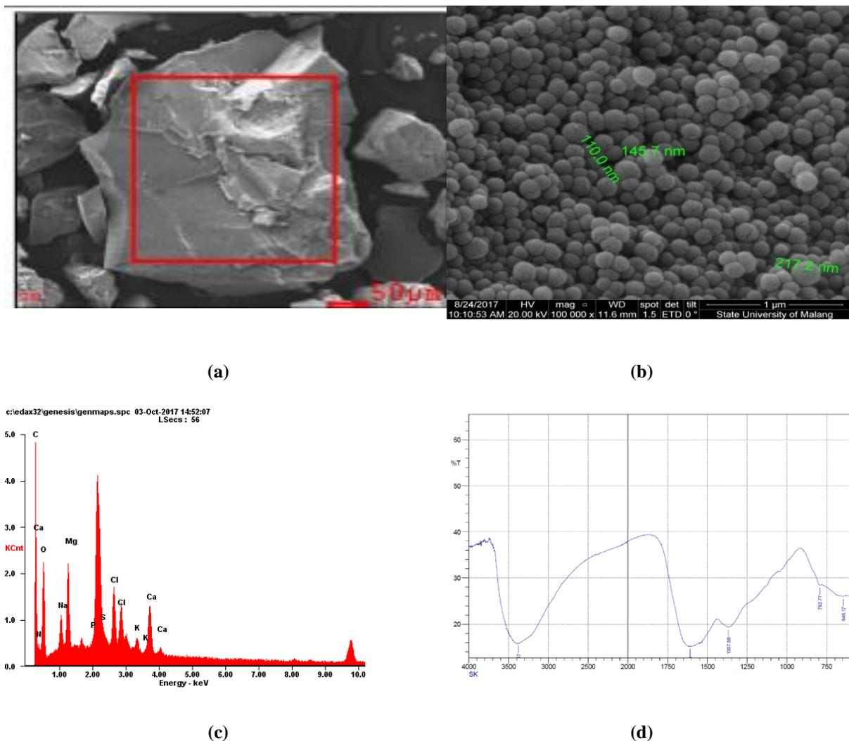
**Fig. 1:** Scanning electron micrograph (SEM) of cuttlefish ink melanin (a) and (b) aggregates melanin, (c) EDX pattern of melanin and (d) The FT-IR spectra of melanin before being purified
