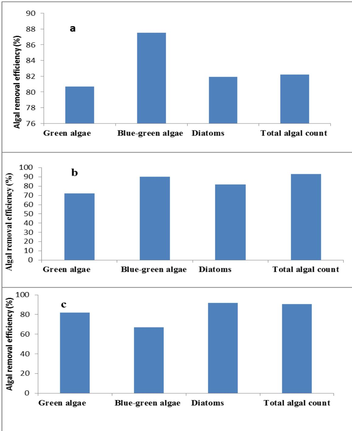
Figure (1) Efficiency of algal removal of using a- Alum, b- FeCl<sub>3</sub>, and c- *Moringa* seed extract
