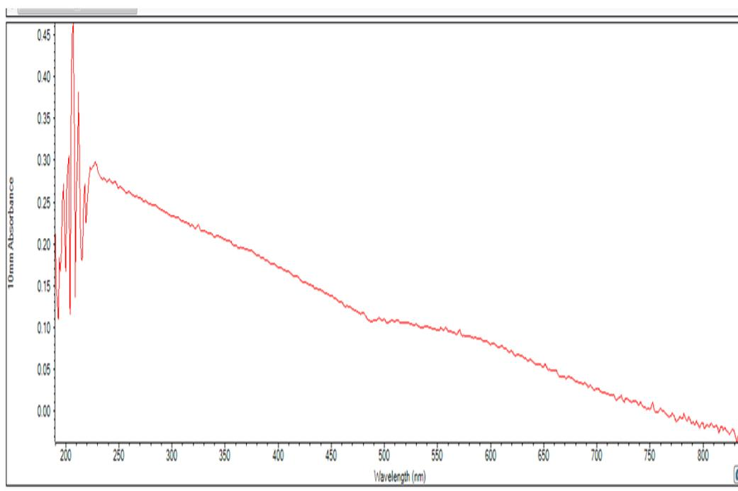
**Figure 1: UV/Vis spectrum of magnesium hydroxide nanoparticles**
