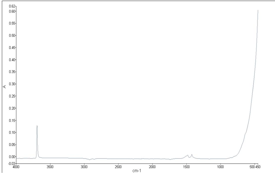
**Figure 2: Fourier transform infrared spectroscopy (FTIR) characterization of magnesium hydroxide nanoparticles**
