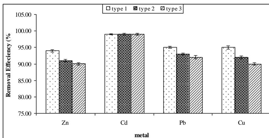
Fig. 3: Effects of chitosan molecular weight on the removal efficiency of metal ions at concentration 20 mg/l
