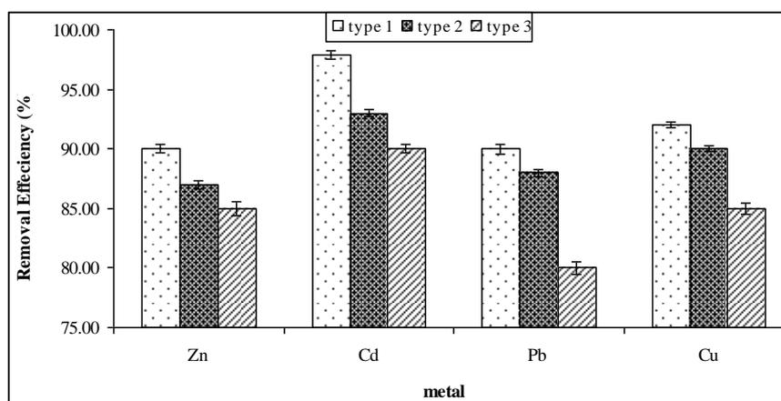
Fig. 4: Effects of chitosan molecular weight on the removal efficiency of metal ions at concentration 30 mg/l
