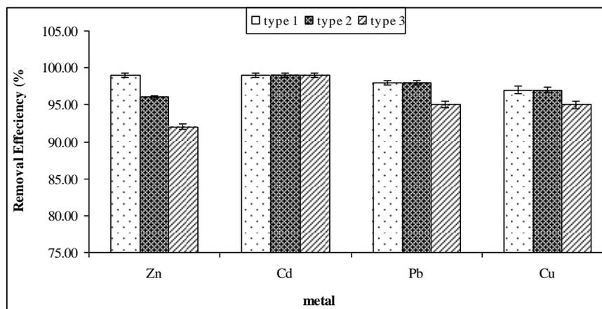
Fig. 2: Effects of chitosan molecular weight on the removal efficiency of metal ions at concentration 10 mg/l
