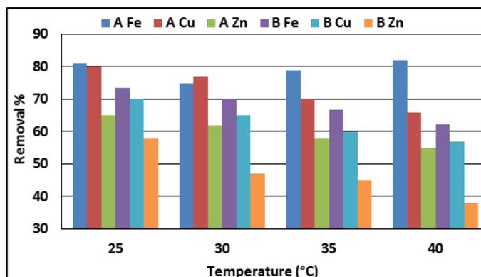
Fig. 9: Effect of temperature on removal percent of heavy metals from wastewater using (A: chitosan) and (B: activated carbon).
