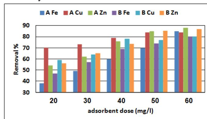
Fig. 6: Effect of adsorbent dose on removal percent of heavy metals from wastewater using (A: chitosan) and (B: activated carbon).
