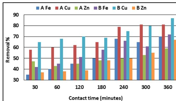
Fig. 8: Effect of contact time on removal percent of heavy metals from wastewater using (A: chitosan) and (B: activated carbon).
