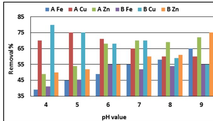
Fig. 7: Effect of pH on removal percent of heavy metals from wastewater using (A: chitosan) and (B: activated carbon).
