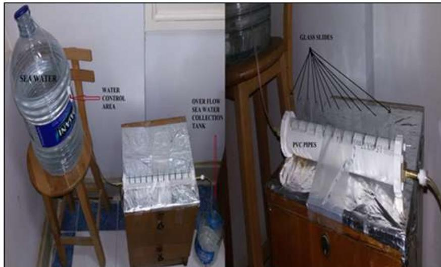
Fig. 1: Biofilm formation device
