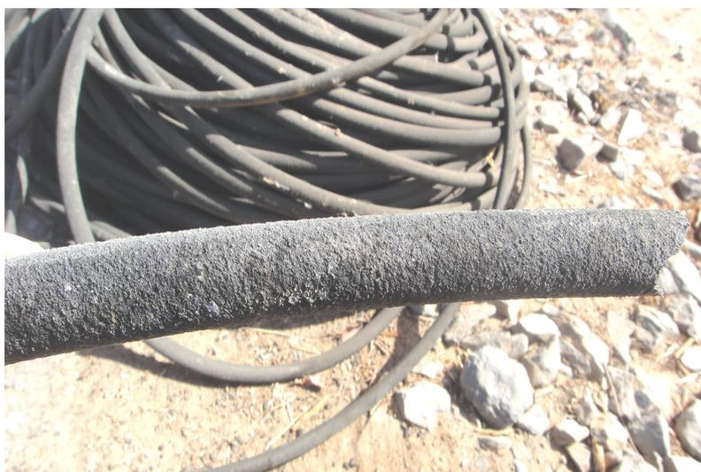
Fig. 2. The subsurface drip leakage lines
