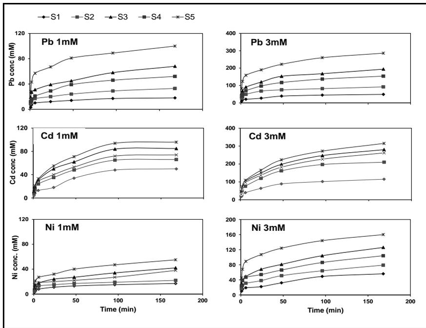
Fig. 1. The concentrations of adsorbed heavy metals on the calcareous soils.
