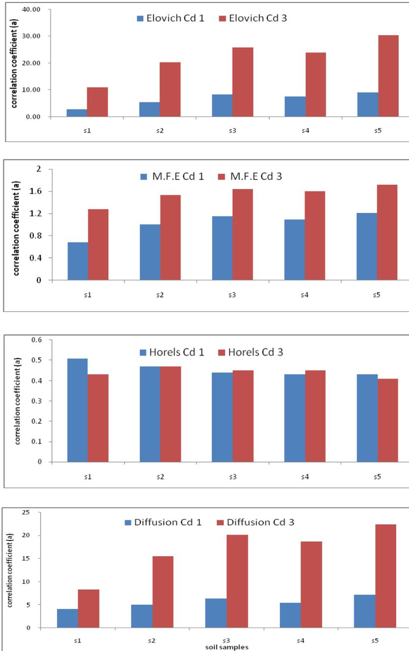
Fig. 3. The correlation coefficient (a) between soil samples and cadmium contents by different kinetics models.
