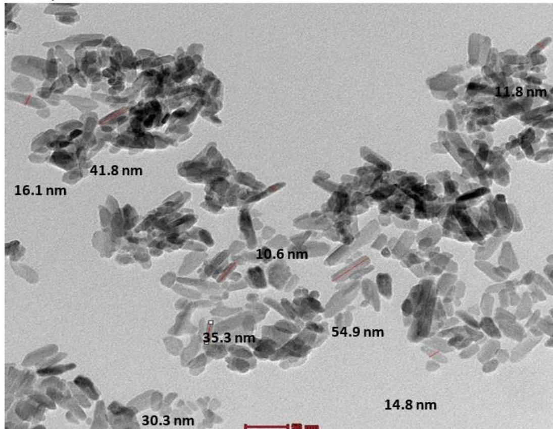
**Fig.2.** TEM image of HA-NPS powders synthesized.
