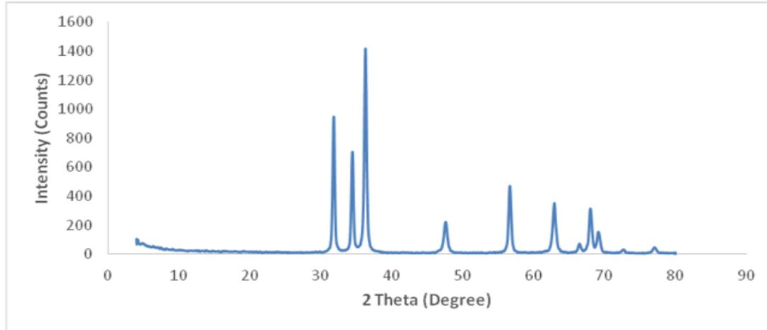
**Fig.3.** The XRD pattern of the synthesized ZnO-NPs.
