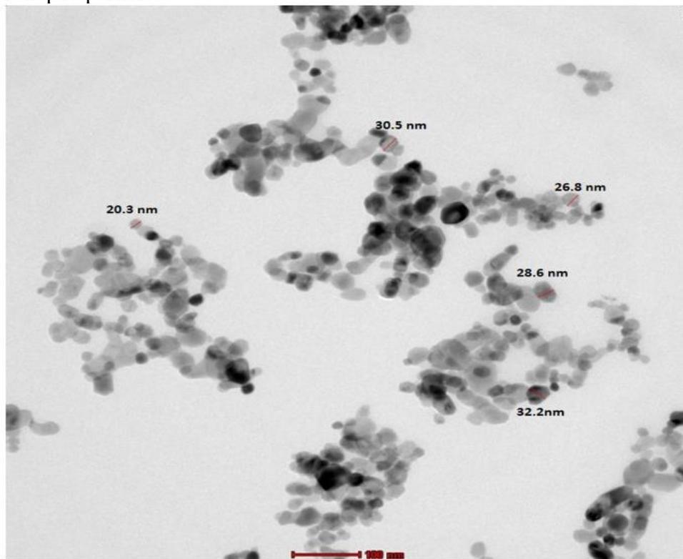
**Fig.4.** TEM image of the synthesized ZnO-NPs.
