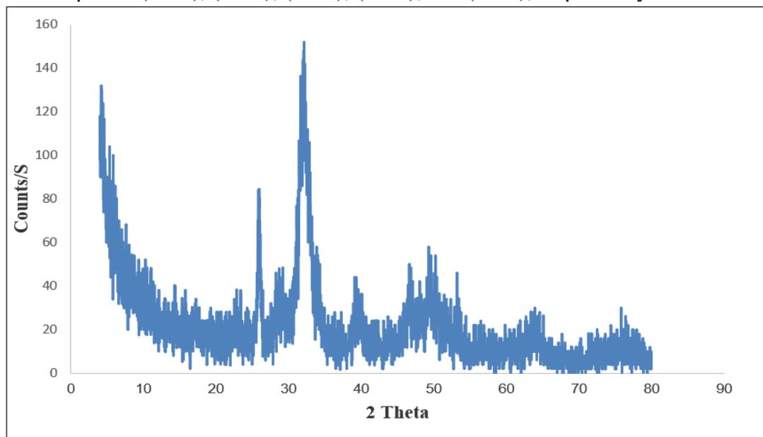
**Fig.1.** XRD patterns of hydroxyapatite (HA) powders synthesized.
