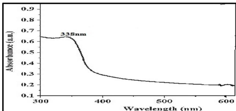
Fig. 3. UV spectroscopy of Nano metal ZnO using Perkin-Elmer S52 Spectrophotometer.
