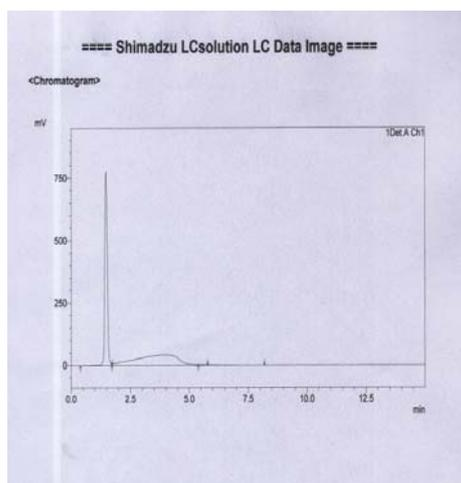
Fig. 1: Chromatogram of imidacloprid standard (1 ppm).
