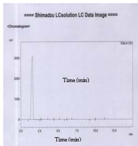
Fig. 2: Chromatogram of imidacloprid standard (5 ppm).
